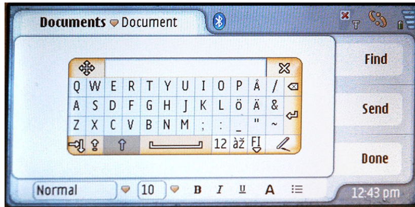
Figure 12 - Nokia 7710 text input method: virtual keyboard as a floating window
